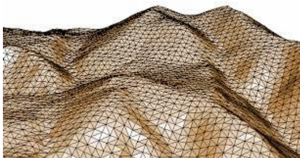
Figure 5: Example of a triangulated irregular network
